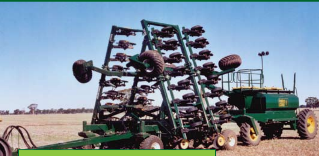
← 12 Metre Single Disc planter on 333mm row spacings and 3 metre tramlines
