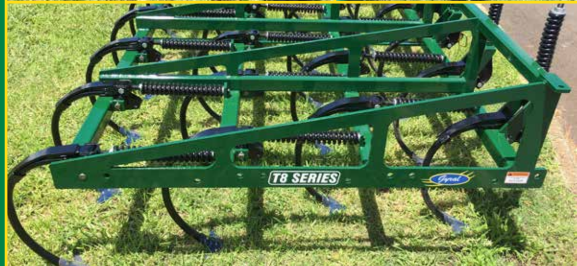
30mm Rounds Solid Tyne 180lbf Breakout
